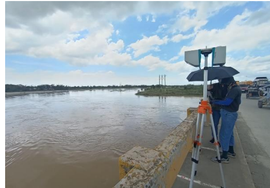
(Pic 43 & 44, L to R) Remains of washed-out houses on the right bank of Peñaranda River along the San Leonardo-Gapan Bridge; and taking surface river velocity of Pampanga River at Vergara Bridge in Cabanatuan City (1312H, Sept 27)
