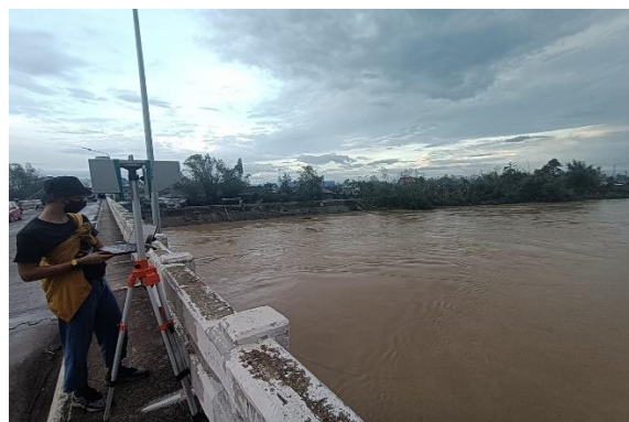
(Pic 48 & 49, L to R) Taking surface river velocity measurements of Pampanga River at Apo Esquivel along the Jaen – San Leonardo Bridge, (1737H, Sept 27); Arayat station's staff gage at 7.98 m, above 6.0 m alarm WL (1100H, Sept 26)
