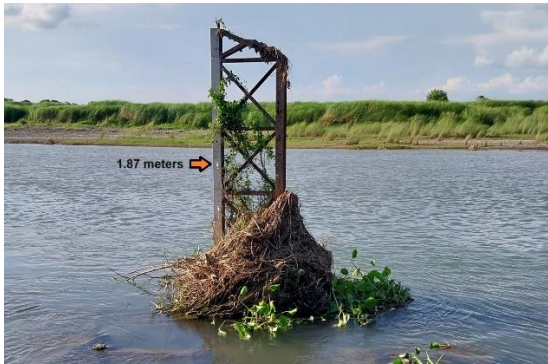
Pic 13 Based on flood marks, the peak staff gage reading at Sapang Buho telemetry station reached around 1.80 meters
