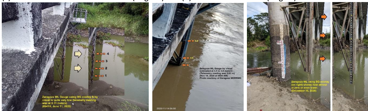
(L) Zaragoza WL at a very low stage (estimated below zero, Jun 11), (Middle) and at an estimated 3.50 m stage (Nov. 14), (R) finally at below zero stage (Dec 18).
