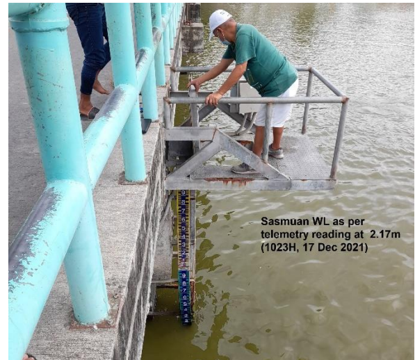
Pic 14 Checking and validating the River WL at Sasmuan stream gaging station on 17 Dec 2021.
