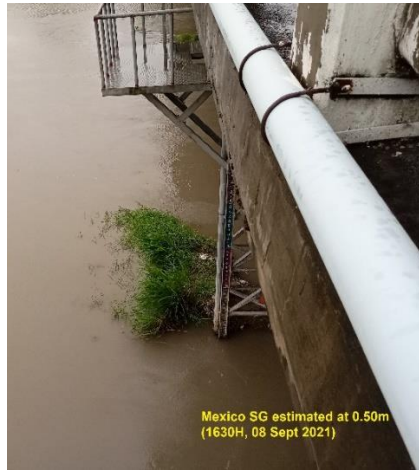
Pic 6 Validation of WL at Mexico staff gage estimated at 0.50m on 1630H, 08 Sept 2021
