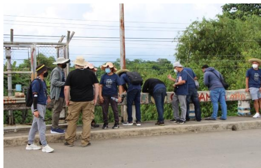
Participants took turns in taking river cross-section by using dropdown line for sounding atop a bridge.
