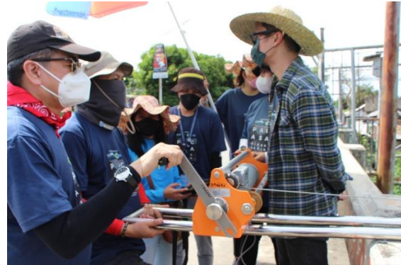
Using a winch with depth counter placed on a bridgeboard was another way of facilitating the measurement of river cross-sections.
