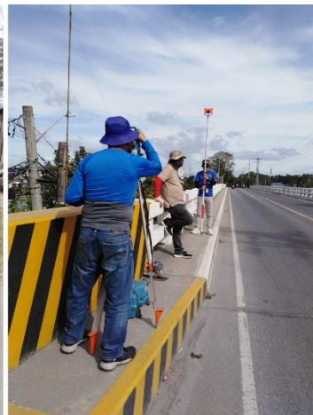
(Pic 26 & 27, above) PRBFFWC and Norzagaray MDRRMO personnel take river sounding atop the Matictic Bridge during the cross-sectioning activities on Feb. 08 & 09, 2023.; (Pic 28, left) River x-sect activities at Sta. Lucia Bridge in Angat, Bulacan; (Pic 29, 30 & 31, below) The same activities at the Plaridel-Pulilan Bridge (left below), and at Bagbag Bridge (middle & right below) in Calumpit, Bulacan.
