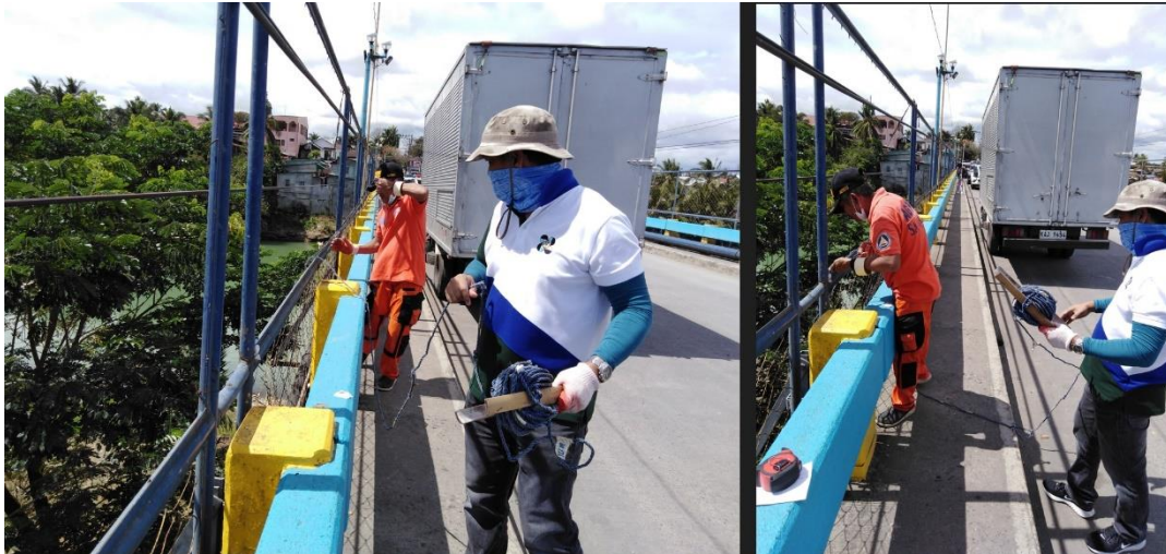
(Pic 26 & 27, above) PRBFFWC and Norzagaray MDRRMO personnel take river sounding atop the Matictic Bridge during the cross-sectioning activities on Feb. 08 & 09, 2023.; (Pic 28, left) River x-sect activities at Sta. Lucia Bridge in Angat, Bulacan; (Pic 29, 30 & 31, below) The same activities at the Plaridel-Pulilan Bridge (left below), and at Bagbag Bridge (middle & right below) in Calumpit, Bulacan.
